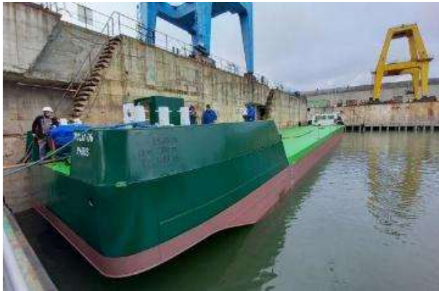
The first self-propelled vessel powered by hydrogen ZULU 06
